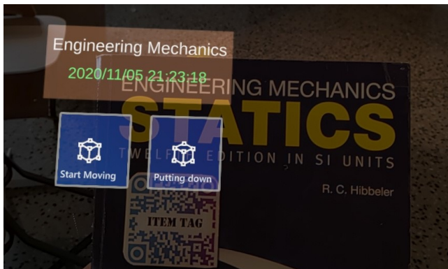
Figure 2: Two buttons and a UI panel are registered on to the fiducial marker when recognised by the Vuforia Engine.
