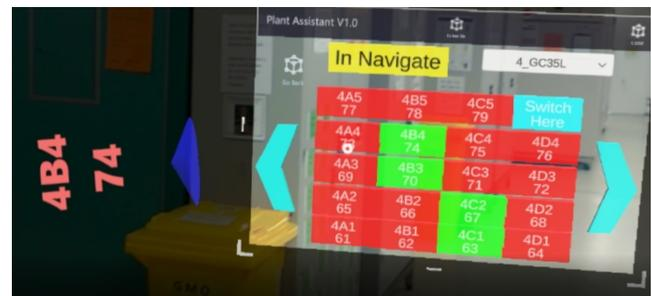
Figure 5: The navigation view—note the blue arrow to the left of the display, which indicates the direction of the particular plant being searched for.
